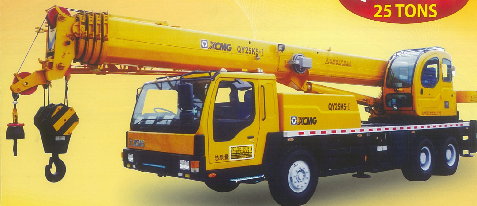
Innovated boom system with inserted sliders, plug-in boom head of patented technology and world advanced shaped boom cross section makes excellent lifting capacity, safe and reliable lifting operations.
