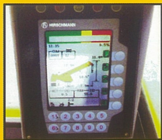
Load moment limiter with color LCD realizes intelligent trouble diagnostic, and its precision leads in the same-class products in the industry.
